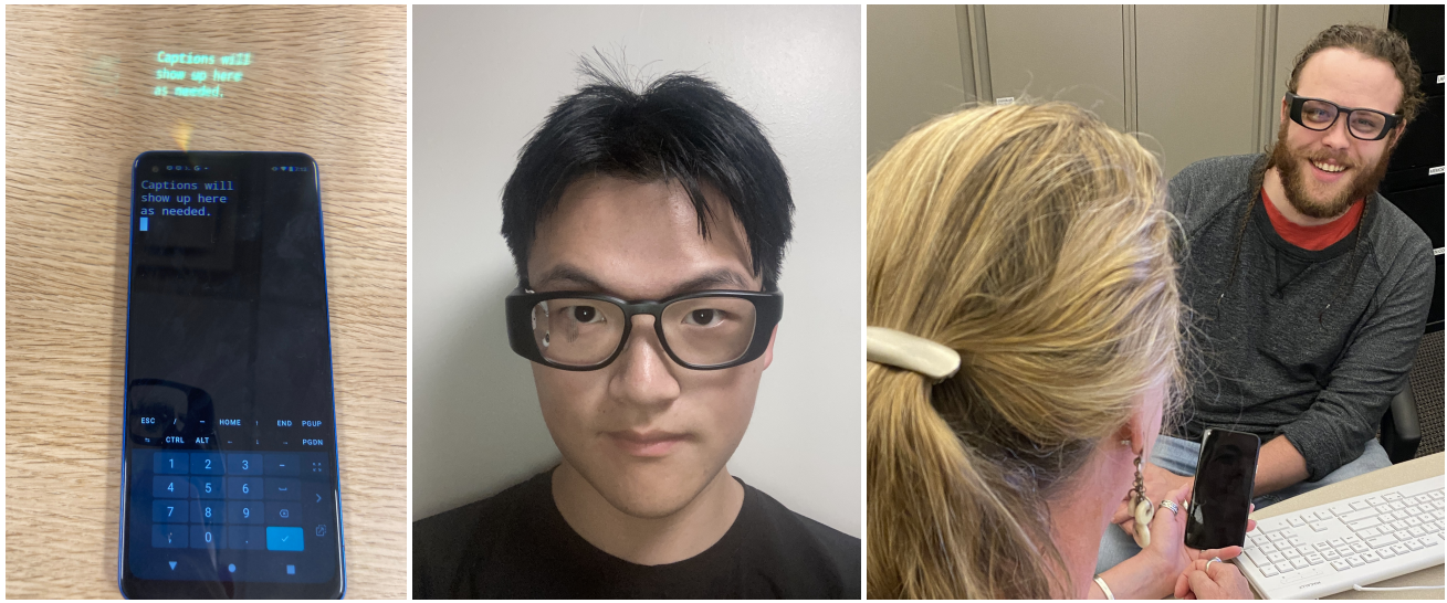
Figure 1: Left: Captions displayed on Android application on mobile phone and on screen of head-worn display. Center: Person wearing tooz DevKit head-worn display. Right: Person conversing using captioning on tooz DevKit head-worn display.
