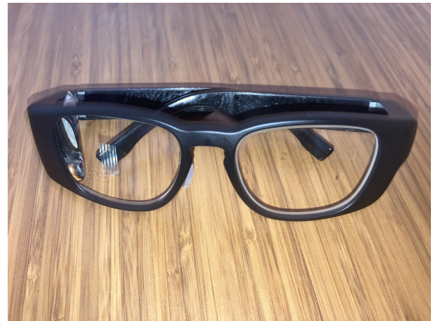
Figure 3: Tooz DevKit Head-worn Display
